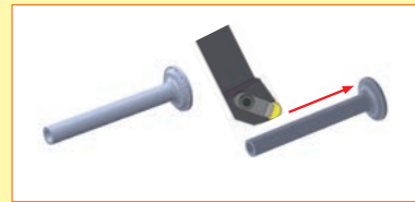
Turbine Shaft RNG 45, 800 SFM, .008 IPR, 080 DOC, WET, Inco 718 (pre-machined)
