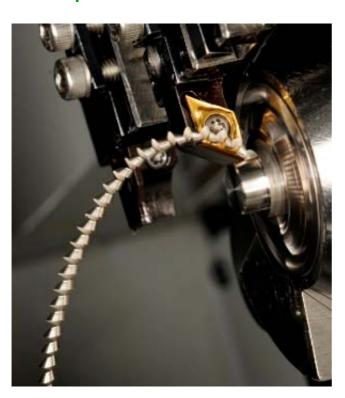
NTK's **CL-chipbreaker** for front turning is an excellent example of our sharp edge technology.
