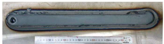
**| What is FSW (friction stir welding)?**
