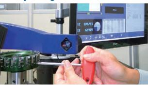
Tighten axial set screw of each insert until you reach around 44.980 mm height dimension. Adjust other inserts within 0.01mm range.
