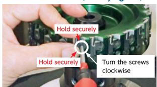
Install the insert to cutter pocket. Tighten wedge set screw with 1Nm torque while pushing insert to cutter center using two fingers. (do not overtighten)
