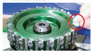
Clean up insert edges using clay.
