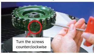
Loosen axial set screw until the screw head is 1 to 2 mm from cutter body.
