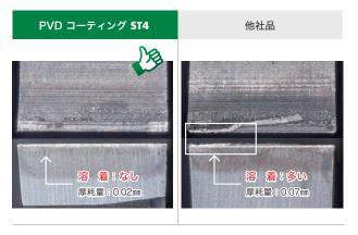
SUS304  $\Phi$ 11  $V_c$ =80m/min f=0.03mm/rev WET , CTPA15FLN
