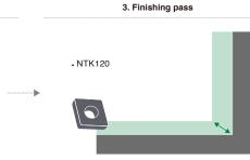
NTK120 - Machine with a consistent DOC to provide stable tool life
