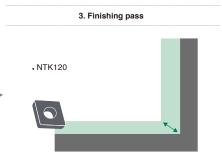
NTK120 - Machine with a consistent DOC to provide stable tool life
