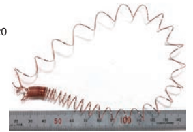
Example of FG chip breaker chips
