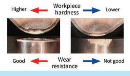
Lower workpiece hardness makes CBN tools wear out easier.
