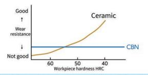
Ceramic has superior wear resistance to CBN in machining workpieces with hardnesses of HRC55 or less.
