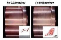
If the cutting conditions cause the chips to become thick (high cutting depth or high feed) then the machined surface will deteriorate due to chip clogging.
