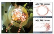
Even if good chip control is obtained at initial stage of machining, sudden chip entanglement can occur leading to tool wear.
