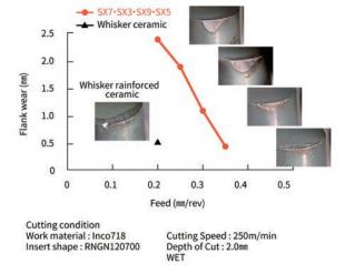
When using the SX7 & SX3 & SX9 & SX5, increased feed is necessary to increase the wear resistance of the tool. By increasing the feed rate and taking advantage of the high tool material strength of the SX7 & SX3 & SX9 & SX5, the number of times the tool and workpiece material rub against each other can be reduced, thereby reducing wear. In addition, higher feed rates shorten cycle time, increasing productivity and profitability.
