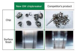
[Cutting conditions] SCM415 groove width: 5.0mm Vc=150m/min f=0.1mm/rev ap=7.0mm No step feed with coolant
