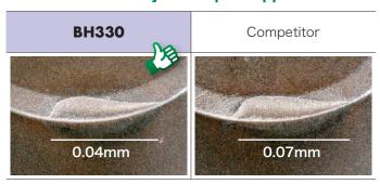
Alloy steel (HRc62)  $v_C$ =150m/min, f=0.1mm/rev,  $a_D$ =0.2mm, After processing 0.7km
